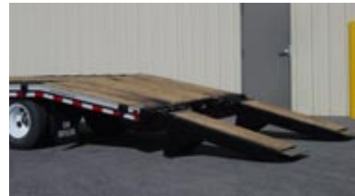
Wood Filled Ramps
