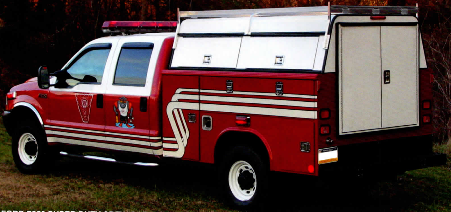
FORD F250 SUPER DUTY CREW CAB WORK BODY HEAVY DUTY COMMERCIAL UNIT WITH A DOUBLE WALK IN REAR DOOR, DOUBLE SIDE DOORS AND A CONTRACTORS RACK.
