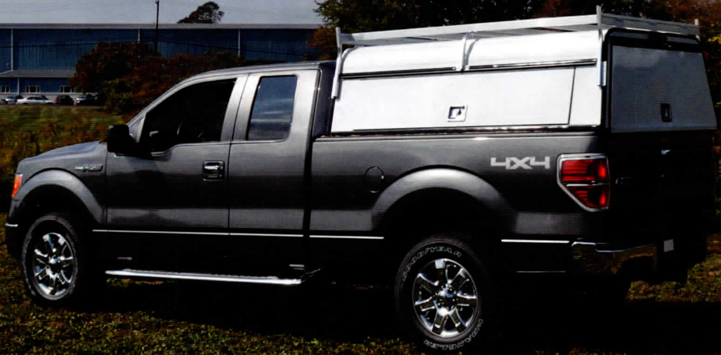
FORD F150 6.5' SUPER CAB 30" HEAVY DUTY COMMERCIAL UNIT WITH SIDE DOORS, A HALF GATE STYLE REAR DOOR AND A CONTRACTORS RACK.
