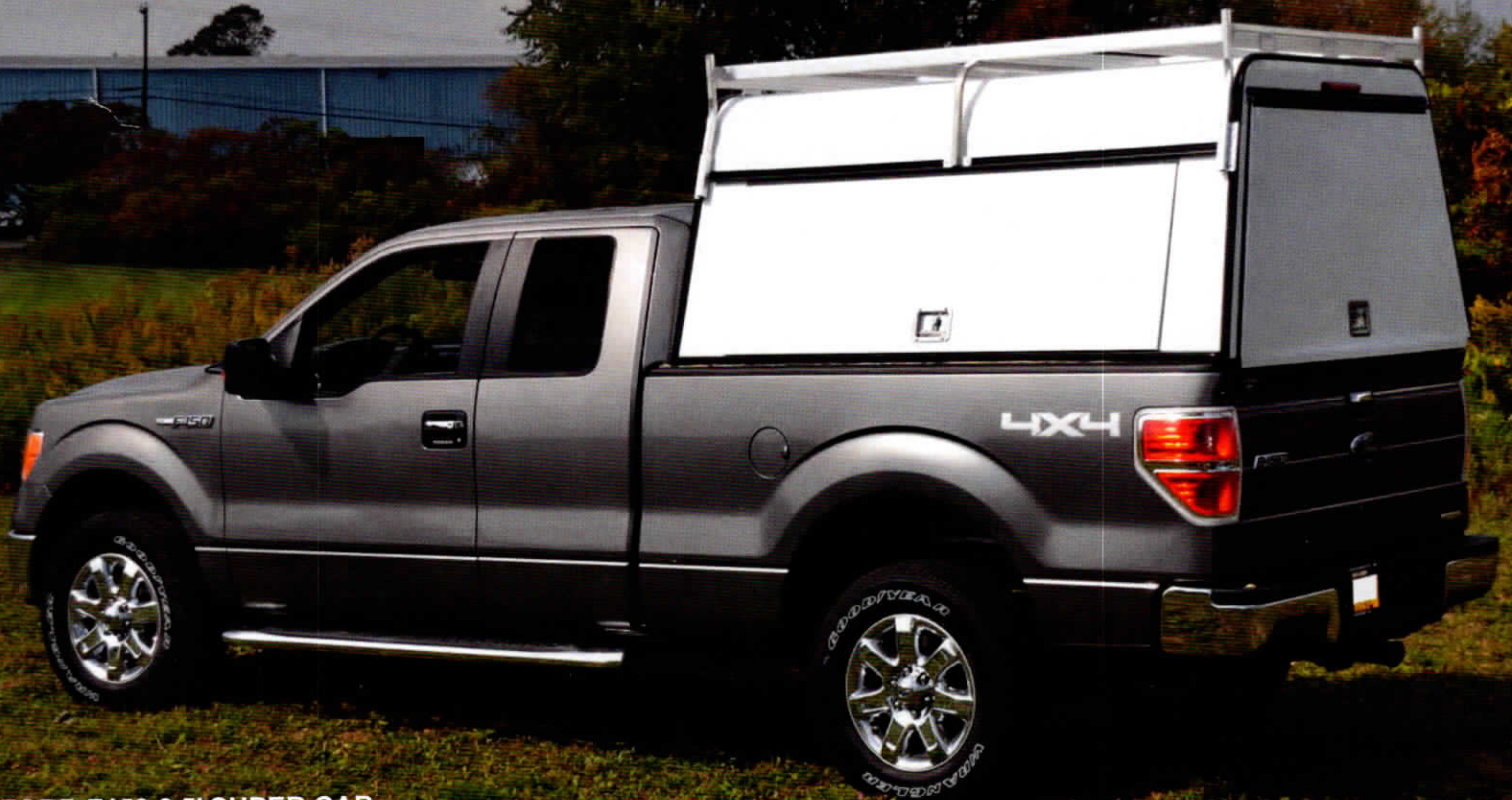
FORD F150 6.5' SUPER CAB 36" TALL HEAVY DUTY COMMERCIAL UNIT WITH SIDE DOORS, A HALF GATE STYLE DOOR AND A CONTRACTORS RACK
