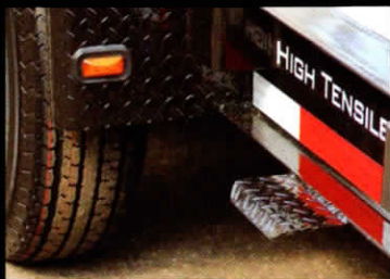
Step To Access Deck
