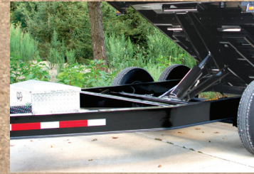
8" I Beam Frame
