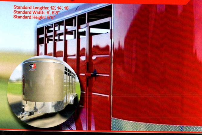
Each bumper stock trailer is equipped with a modern low profile roof, sleek crimped steel sheets, extra tubing supports on rear and center gates to provide extra support, and treated plank flooring. S&S applies a high-solid poly-urethane PPG paint to each of its trailers for the best shine and for scratch resistance. Every trailer is hand made with the customer in mind.
