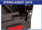
Our durable springs help you raise and Heavy-Duty square tube construction for lower your ramps more easily and safely proven durability. Folds flat to reduce air resistance.
